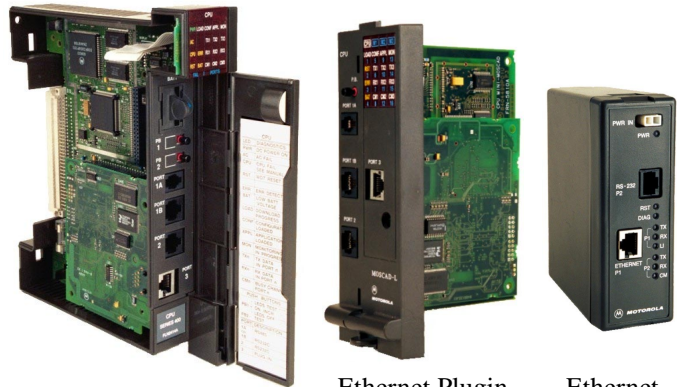
Ethernet Plugin in MOSCAD CPU
